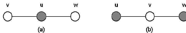
Fig. 7. (a) Node u is in Independent Set (b) Node u and Node w are in Independent Set
